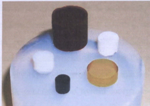
Figure 2.1. Different type of transition metal oxide aerogel (AEROGEL.ORG, 2018).
