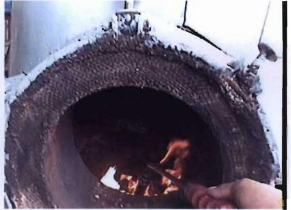
Figure E6: Feedstock ignited inside pyrolysis chamber
