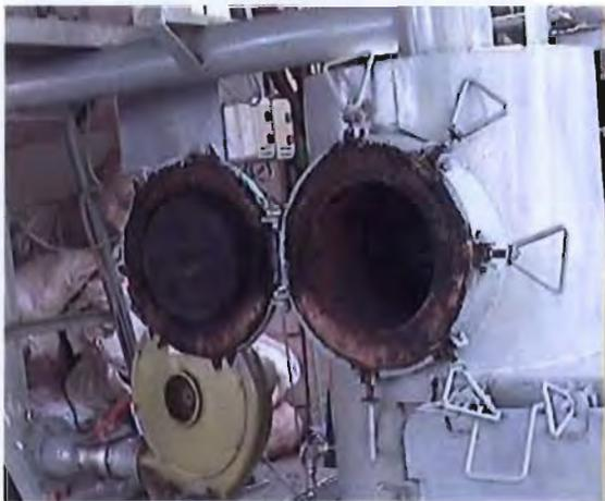
Figure 5.8: A view of pyrolysis chamber
