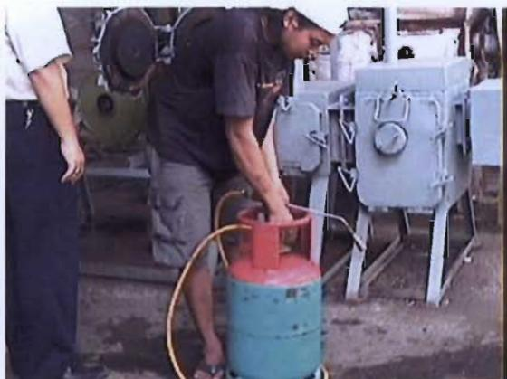
Figure E4: Natural gas being used as ignition starter
