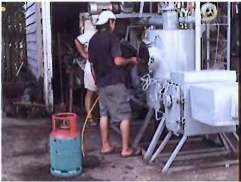
Figure 5.14: Initial ignition of feedstock in pyrolysis chamber
