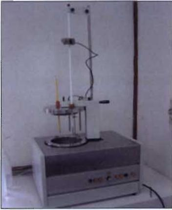
Figure 3.3: Bomb calorimeter
