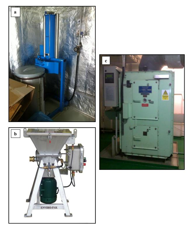
Plate J-3: Garbage processing equipment available on the vessel including (a) compactor, (b) comminutor and (c) incinerator.
