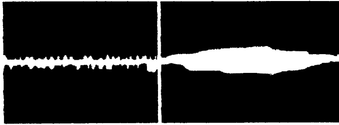
A. Surface roughness; B. Poor surface flatness
