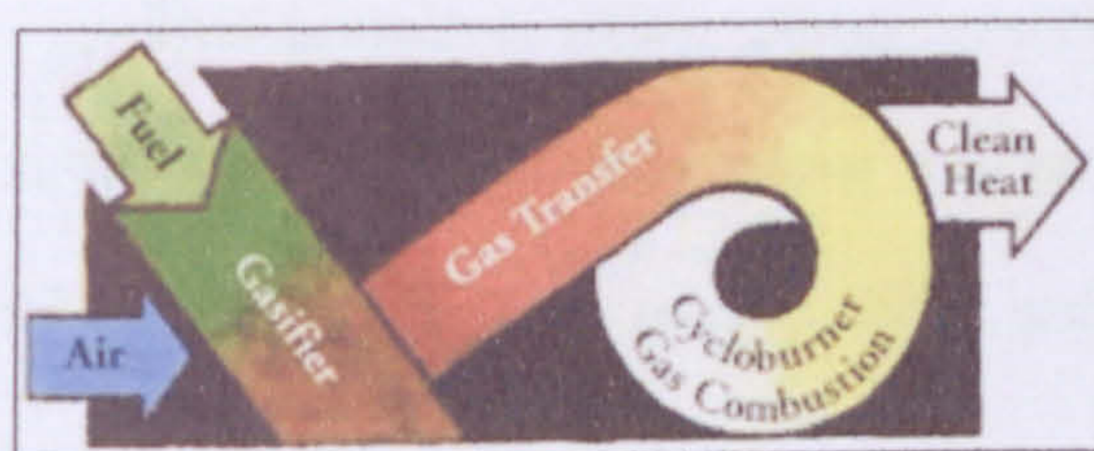
Figure 1.2 Illustration for gasification process.
