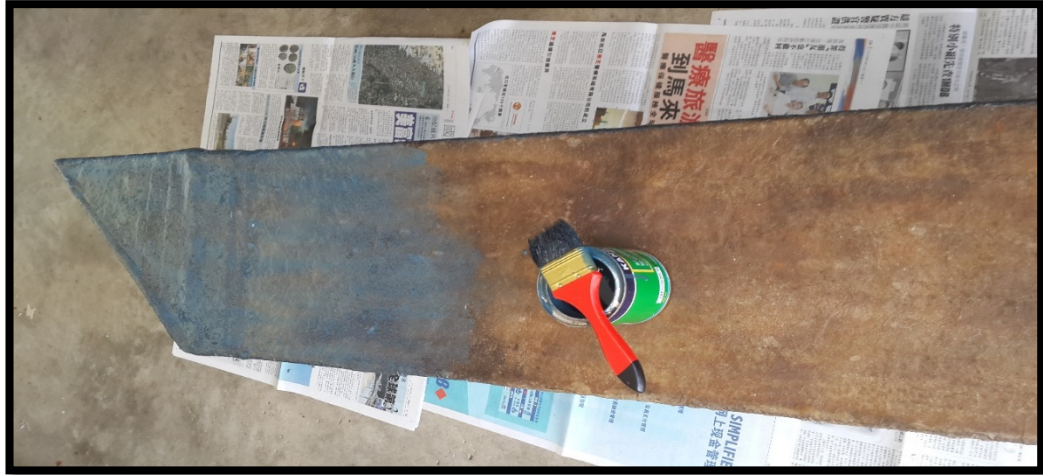
Figure 3.12: Painting the Fiberglass Float
