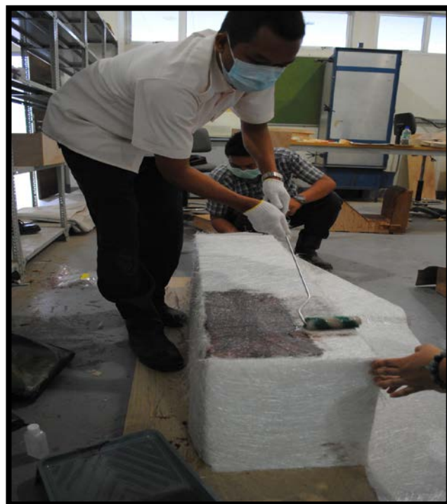
Figure 3.11: Applying Resin to the First Layer of Fiberglass Cloth
