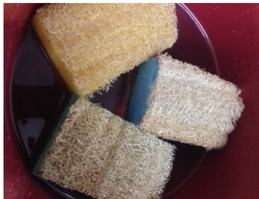
Figure 5.11: Luffa fiber attached to sponge are soak in water for several days
