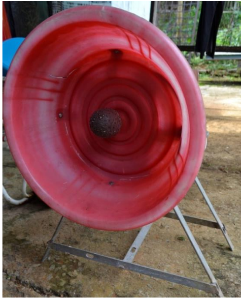
Figure 4.24: Coconut grater made from washing machine dynamo and plastic basin
