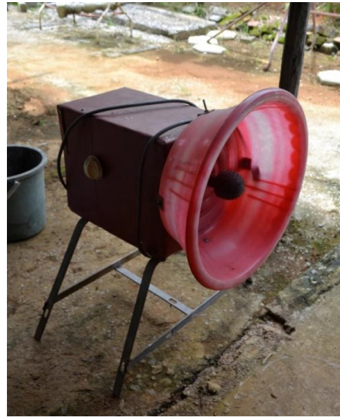
Figure 4.24: Coconut grater made from washing machine dynamo and plastic basin
