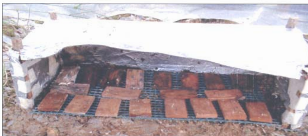
Plate 1: Woods that place on netlon mesh exposed to the environment.
