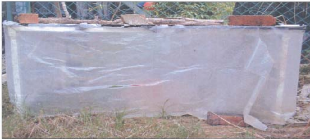
Plate 2: Modified field technique to place the woods at natural exposure.
