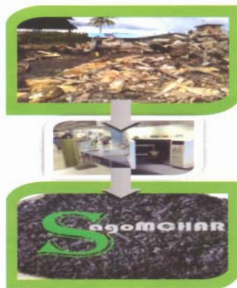
Figure 1. Sago bark waste was converted into biochar (SagoMChar) via microwave carbonization
