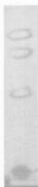
Figure 4: The spots of triterpenoid acids from extracellular in solvent system methanol: hexane (1: 0.5)
