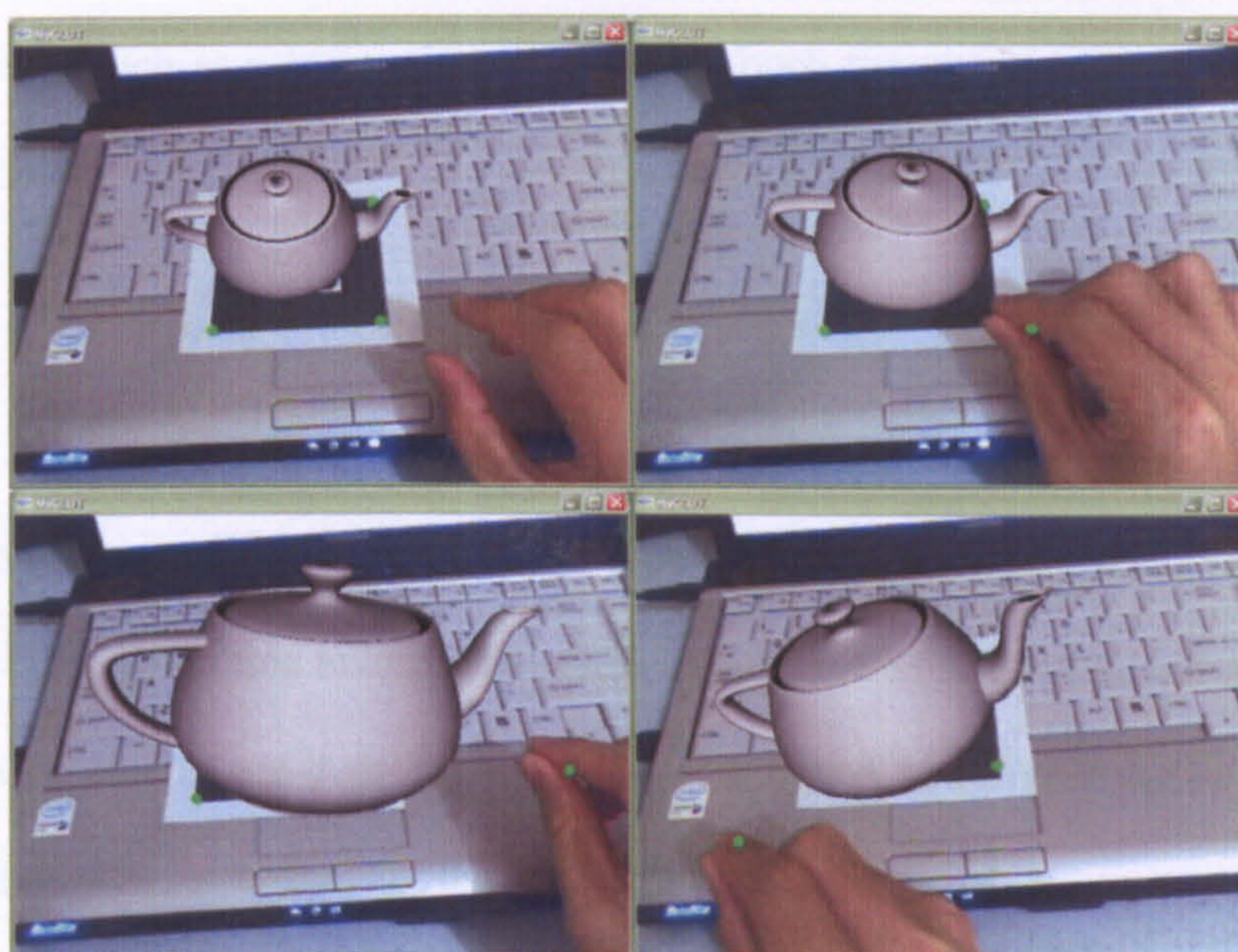
Figure 5.15: Screenshots of finger tracking as an input device for interaction in AR system.
