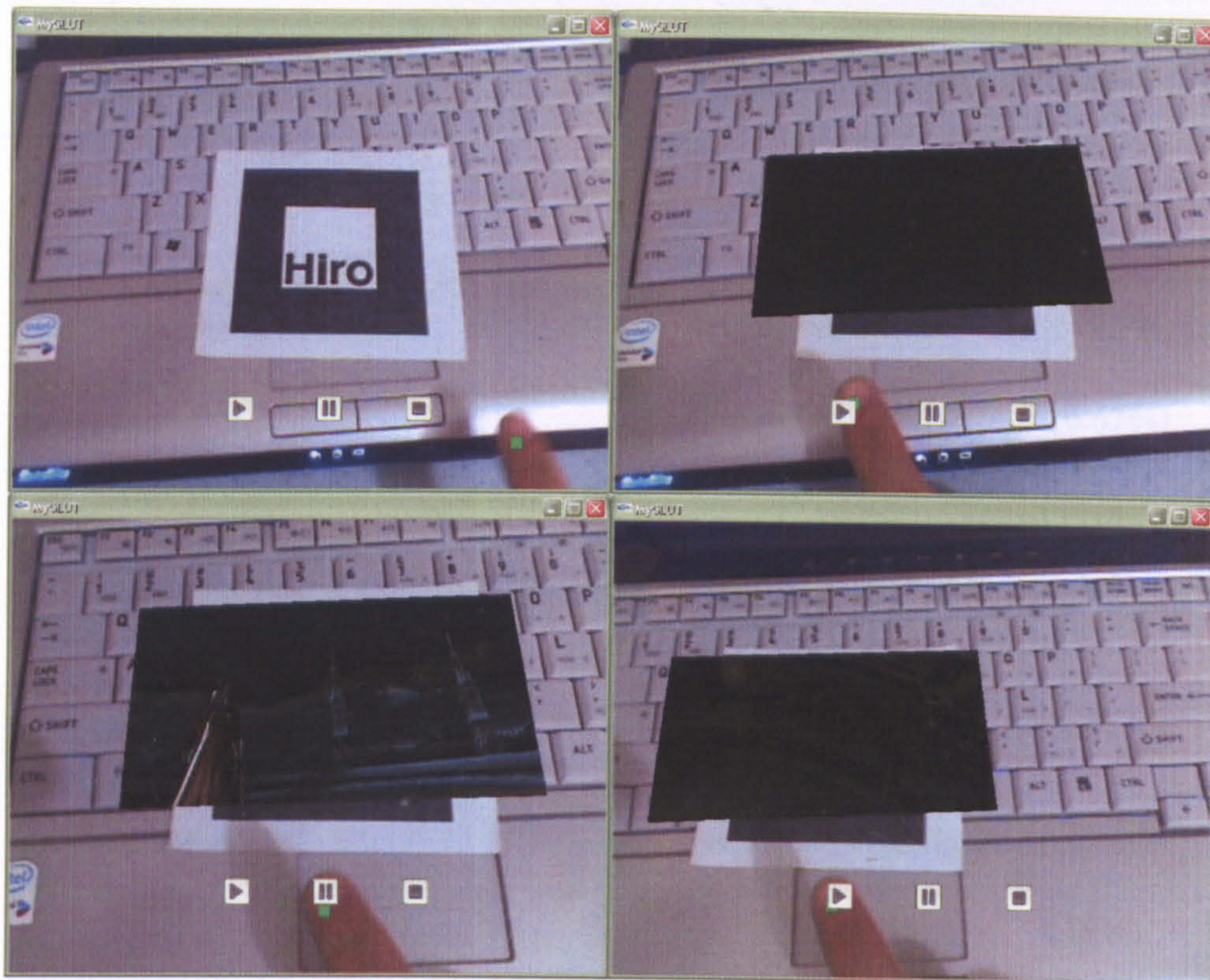
Figure 5.16: Screenshots of AR video player and using finger as an input device to operate the virtual player.
