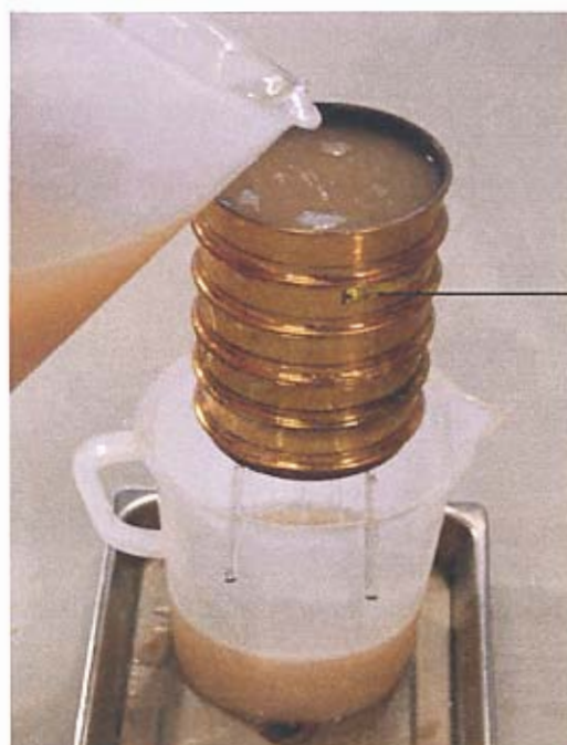
Figure 2: The sago effluent filtration process.
