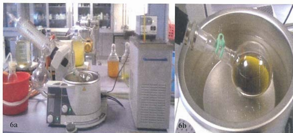
Figure 6a & 6b: Vaporization of hexane from the lipid extracted using rotary evaporator.
