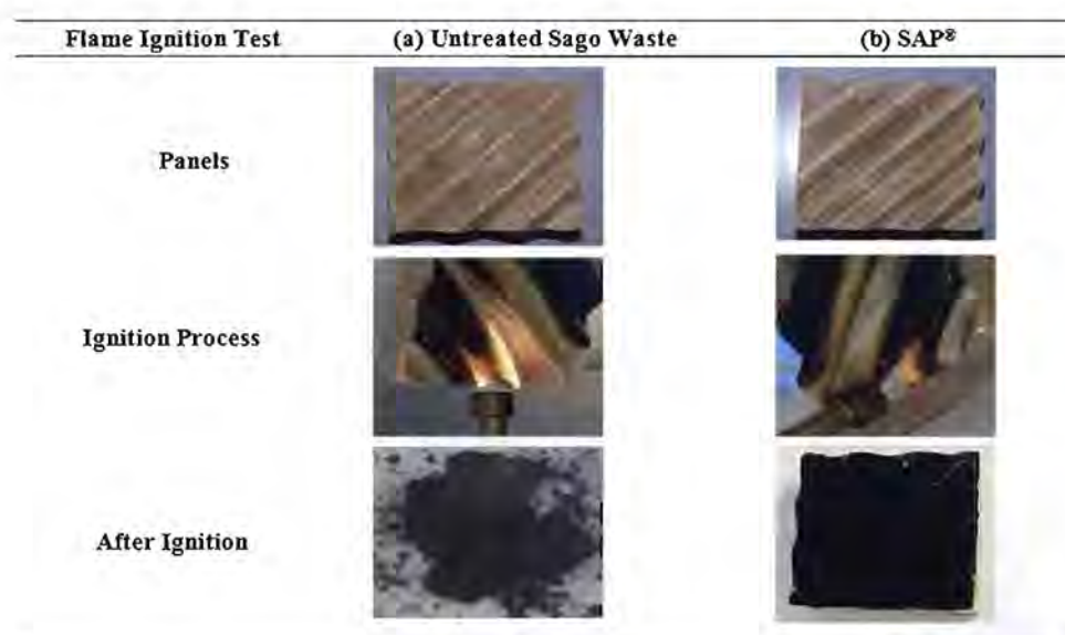
Figure 1: Flame ignition test of (a) Untreated Sago Waste (b) SAP®.
