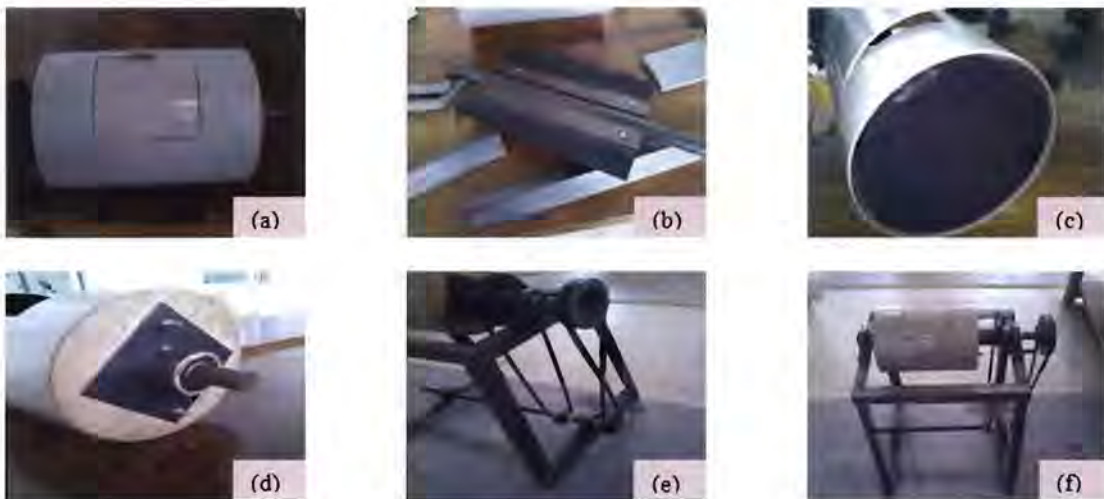
(a) Main body (b) Blade (c) Inner cylinder (d) Side cover (e) Shaft, pulleys, gears (f) Assembled figure of retting machine.
