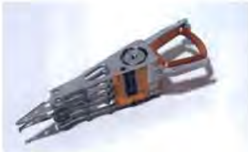
Actuator arm in HDDs.
